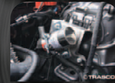
Engine Bay Fire Suppression System
